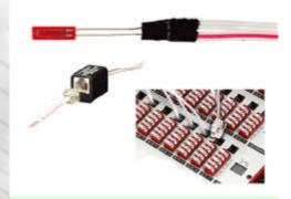
TML have introduced a new 4-wire single strain gauge system that solves the problem of temperature changes due to lead wires, and also any contact resistance effects when connectingup the gauge to instrumentationorin-line connections. This enables long thin cables to be used with low cost connectors.
