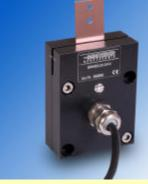
A unique product in the Schreiber Messtechnik range of inductive displacement sensors, is their model SM48slotsensor. Insteadof the standardofferingof extending shaft sensors, these devices measurethe position of a thin vane passing through a slot in the sensor
