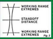
Common sensor design practice is to focus the laser beam to create the smallest spot at the sensor standoff distance. This is the point where the laser spot size is specified. The size of the beam is then smallest at the standoff point, but it is larger both inside and beyond this point (Figure 2). Where the smallest spot size is required, the Fig. 2 sensor will perform best for objects near the stand-off (best focus). Triangulation
