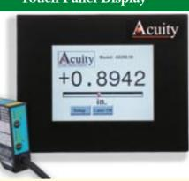
New to the Techni Measure range are the laser displacement sensors from Acuity. The triangulation sensors can be used in pairs for measuring the thickness of a target, and the new 5.7" touch panel display offers simple setup to give a direct display of the thickness of a target that is put between these two sensors. The meter can also be used with a single sensor, in order to display measurement data from most of the Acuity range of sensors.
