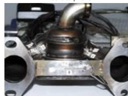
High temperature weldable strain gauges fitted to an engine manifold.
