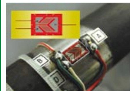
Special chevron type strain gauge for torque measurement
