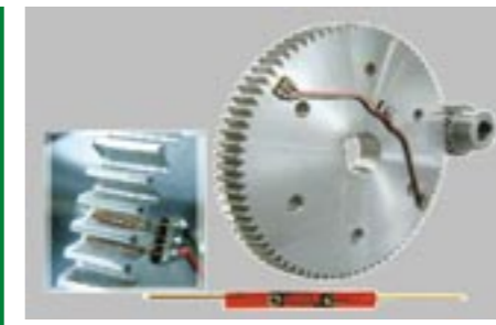
Miniature strain gauge fitted in the valley of a gear tooth
