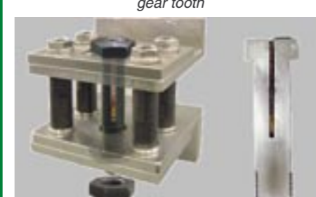
Bolt strain gauge fitted into a bolt for axial measurements
