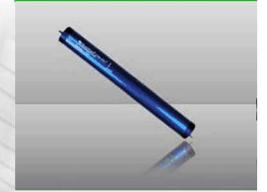
The MicroStrain 3DM-DH3™, is a downhole orientation sensor and datalogger. It incorporates acceleration sensors, magnetic field sensors, and temperature sensors, together with an on-board microprocessor, embedded software algorithm, non-volatile memory for configuration, flash datalogging memory, and a serial communication interface. Its form-factor, rated temperature range and power supply requirements are optimized for downhole applications.
