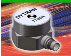
Dytran Instruments have just released a new version of their high performance, variable capacitance (VC) accelerometer. The 7700A series is a family of DC response accelerometers that were designed, utilizing a capacitive sensing element and an advanced ASIC, to simulate the operation of a strain gauge bridge in order to directly replace piezoresistive units in new or existing applications, but they also have the same form factor as a standard piezoelectric
