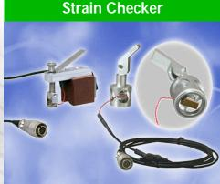
TML have introduced another new design of holder for their frictional strain gauges. The new FGMH-1B and FGMH-2A are designed for metallic targets, since a magnet holds the Strain Checker to the structure whilst a spring holds down the integral frictional gauge to the surface.
