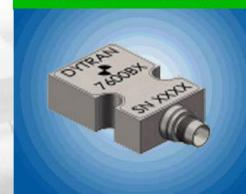
Dytran Instruments have just released a new technology of high performance, variable capacitance (VC) accelerometers. The 7600B series is a family of DC response accelerometers that were designed, utilizing a capacitive sensing element and an advanced ASIC, to simulate the operation of a strain gauge bridge in order to directly replace piezoresistive units in new or existing applications.
