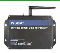
The new WSDA® unit from MicroStrain is a ruggedised, single board computer with Ethernet and optional cellular connectivity, designed to collect data from networks of wireless sensors. The WSDA® is compatible with all MicroStrain wireless sensor nodes and can collect and store up to 2GB of data locally.
