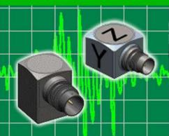
Dytran have recently introduced several new triaxial accelerometers. In particular the models 3333A and 3363A offer miniature size with low noise outputs. Both are IEPE type sensors and available with sensitivities of 10, 50 or 100mV/g, but the 3333A are adhesive mount, whereas the 3363A are stud mount.
