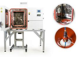
acceleration sensor according to ISO 16063-21, where the vibration exciter with reference sensor is integrated into a temperature chamber. Thus, it is possible to calibrate not only at room temperature but over the entire temperature range mentioned
