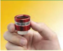
TML have introduced a novel device for applying pressure to a strain gauge, whilst the adhesive is setting during installation. The magnetic Pressee with a built in magnet, part number PM-19, can be used on appropriate flat metal specimens over 1mm thick, is very easy and quick to apply, and also allows for the gauge placement to be viewed through the clear view central area.
