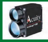
own signal. The time that the light takes to travel to the target and return, plus the time needed to amplify the signal, determines the period of oscillation, or the rate at which the laser is switched on and off. This signal is then divided and timed by an internal clock to obtain a range measurement. The measurement is somewhat nonlinear and dependent on signal strength and temperature, so a calibration process is performed in the sensor to remove these effects.
